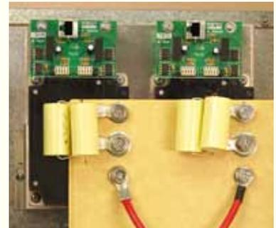
The generator uses Pulse Width Modulation to control the input power of the HV Transformer to develop and maintain the proper output. This Pulse Width Modulation allows for the precise adjustment of tube current and kVp during the EXP Cycle. Power line deviations of up to +/- 10% can be compensated for automatically using Pulse Width Modulation.
