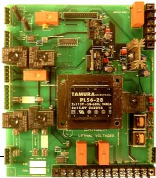
The incoming power is fed through the line fuses to the input connector on the SPB circuit board.
